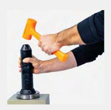
It allows the mounting of bearings of different sizes, starting from small calibers to large calibers. With the help of the recoilless hammer included in the set, the hammering process is both facilitated and occupational safety is ensured.
