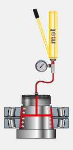
This method is generally used to remove bearings that have been mounted using a hydraulic nut. High forces are required for dismounting large caliber bearings. A hydraulic hand pump is used to achieve high power without any serious effort. With the help of this pump, which can be pressured up to 700 bar, it is possible to obtain large forces and easily remove the bearings.
