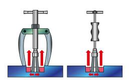
The internal pulling method is used in applications where the bearing can only be held by its inner ring. The diameter range varies depending on the size of the pulling collets inside the internal drawing module. Each collet in the module can be adjusted according to the desired diameter between two minimum and maximum values. With the help of this method, which is not known and frequently used in the industry, dismounting can be done without damaging the bearing.
